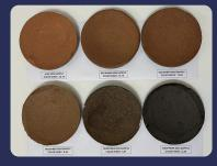
Natural Pozzolan Replaces Clinker 'Cape Verde,' which means 'Green Cape' in Portuguese, possesses abundant natural pozzolan resources. When used as an alternative to clinker, for example, in CEM II 42.5 type cement, it can replace traditional clinker, which emits 750-800 kg of CO<sub>2</sub> per metric ton, with zero carbon emissions per metric ton, of pozzolan.
